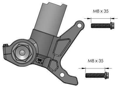
Use your motorcycle's original (OEM) M8 x 35 mm bolts to mount the caliper adapter bracket.
