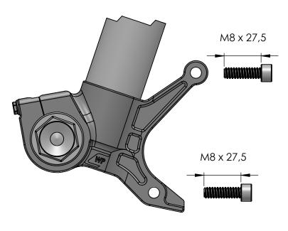
Use the included Moto-Master M8 x 27.5 mm bolts to mount the caliper adapter bracket.
